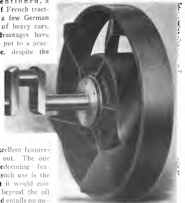
Fig. 18.—Efficient arrangement of both fan and flywheel in a unit.
